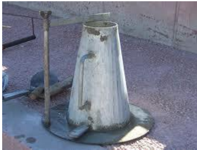
Figure 5.1 : Slump Testing Apparatus
