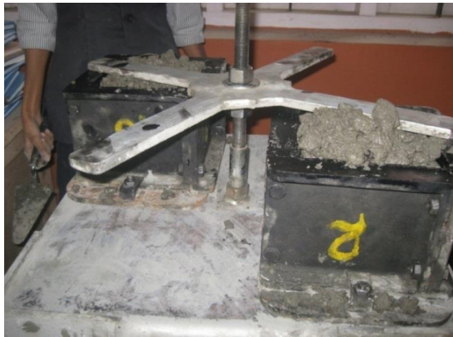
Figure 5.3.2.1(b) : Cubes Specimen Placed on Table Vibrator
