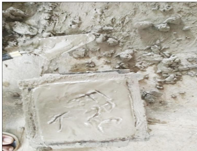
Figure 5.3.2.1(d) : Finished fibre reinforced concrete cubes
